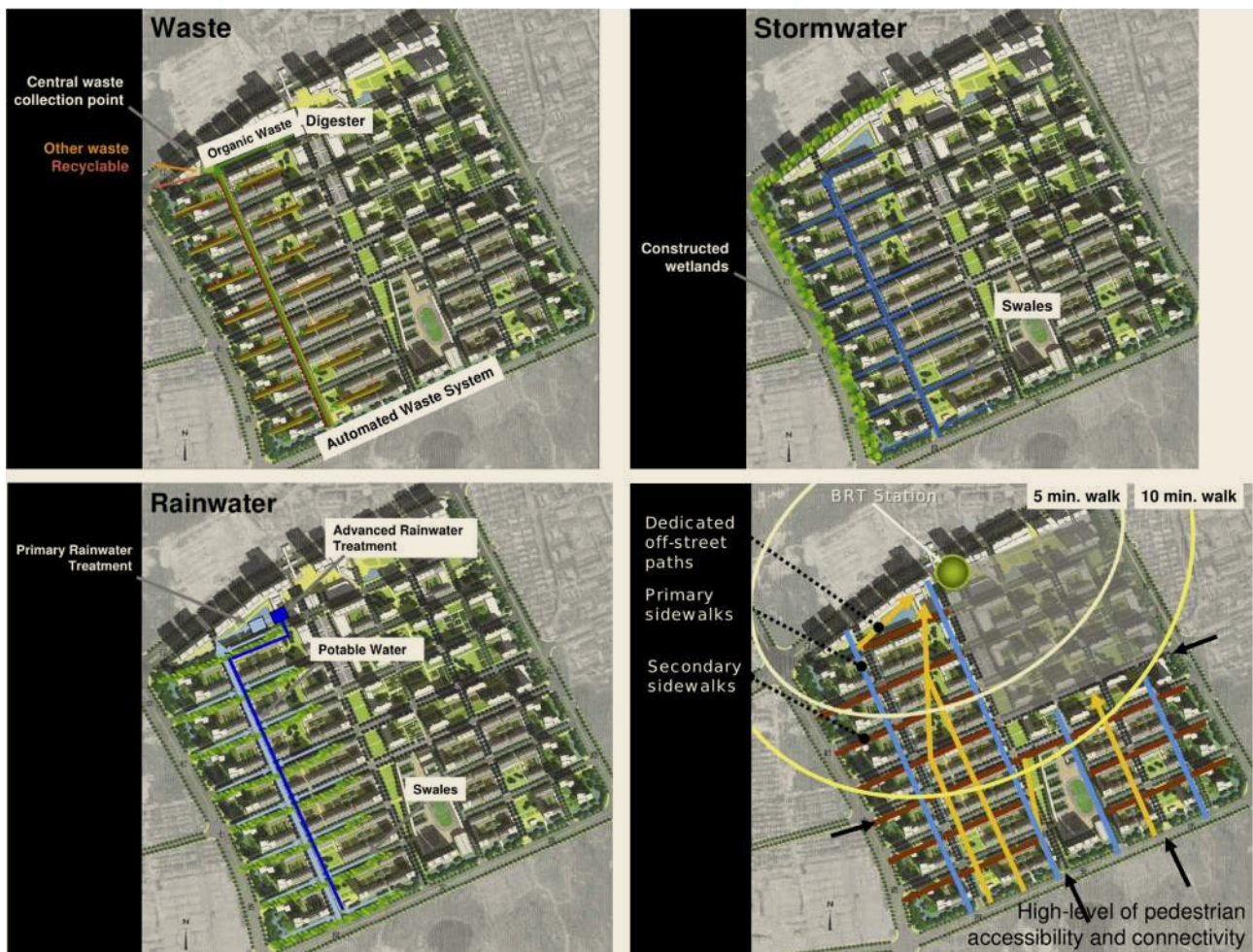
FIGURE 4.9 INFRASTRUCTURE SYSTEMS LAYOUT.
