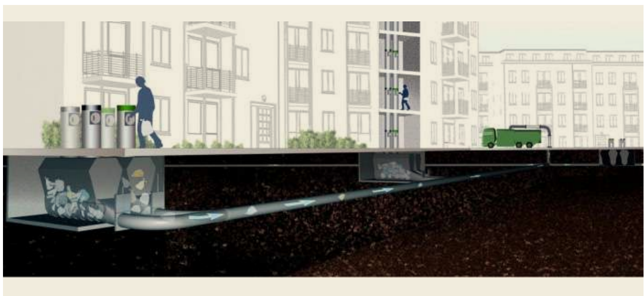
FIGURE 4.11 UNDERGROUND WASTE COLLECTION SYSTEM (SOURCE: GRANATIERO 2014)
